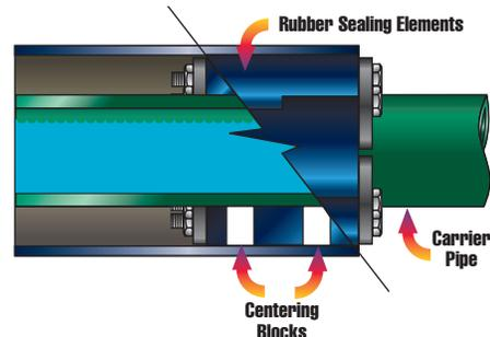
\*Centering Blocks are plastic reinforcements that assure a penetrating pipe will stay "centered" within its casing and adds extra support against heavy loads from back fill.
