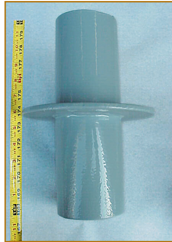
Figure 1: Gal-vo-plast ® Wall Sleeve submitted for testing
