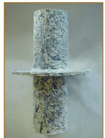
Figure 4: Galvanized Wall Sleeve after 500 hours of exposure
