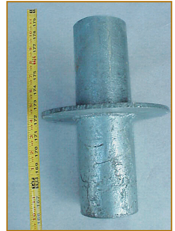
Figure 2: Galvanized Wall Sleeve submitted for testing
