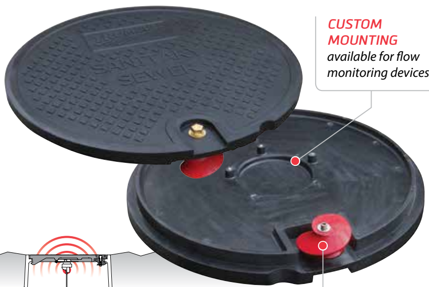
WORM GEAR secures lid to frame and is operated with a bronze pentagon bolt; other locking options available upon request
