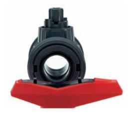
The Type 546 Ball Valve seat carrier is reverse threaded while the valve nut utilizes a standard thread. This ensures that the seat carrier is not inadvertently tightened when the valve nut is tightened and avoids possible stem failures.
