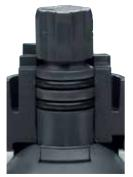
The Type 546 Ball Valve stem utilizes a predetermined break point opposite the media side of the stem seals. This break point is a groove with an inner diameter that is less than the stem seal grooves. This ensures that if there is a stem failure, the failure will occur at that point and media will not leak to the outside of the valve.
