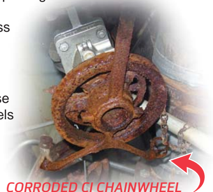
CORRODED CI CHAINWHEEL shows advantage of stainless
