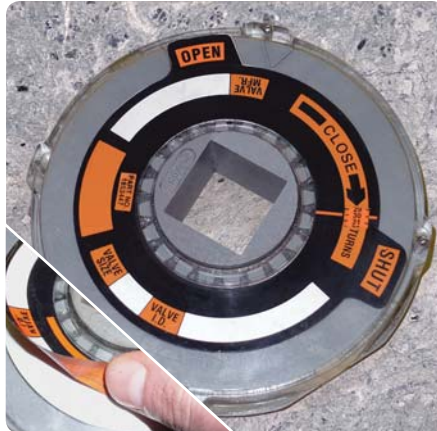
Adhesive labels can peel off in high temperature or humidity.
